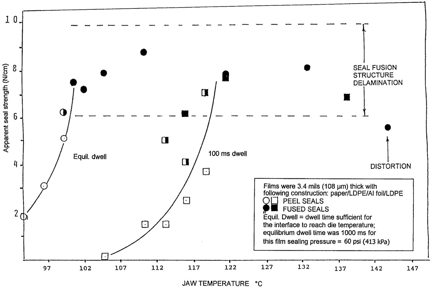
FIG. 3 Heatsealability Test Method Example
